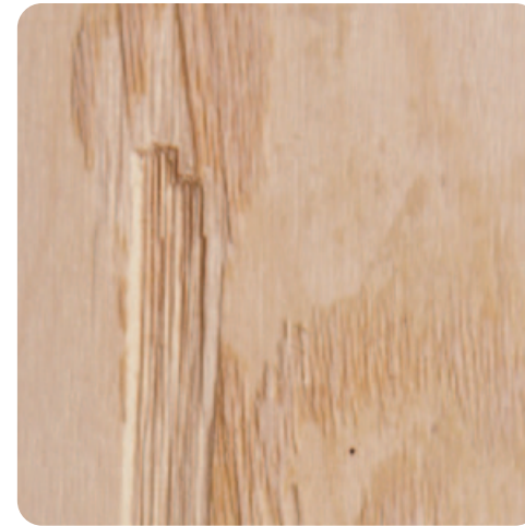
Breaking out of grain
