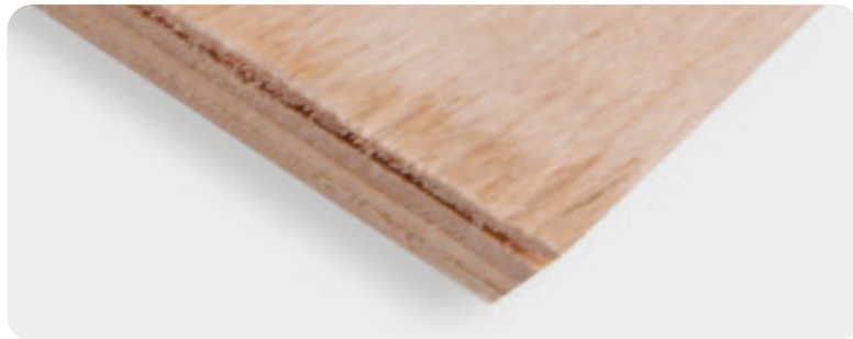
Veneer shortage in the inner layers
