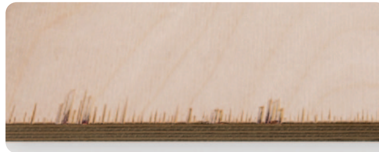
Shatters (defect due to cutting)
