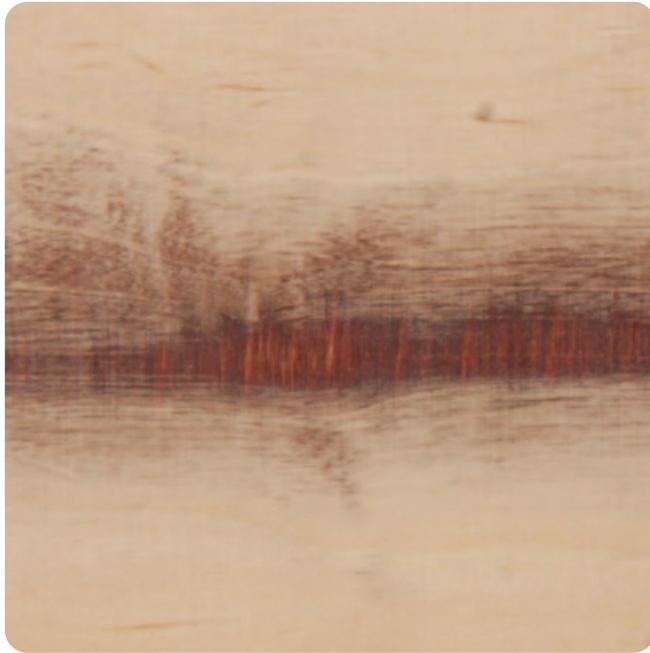
Grinding on MR-glywood
