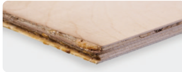
Shatters (defect due to cutting)
